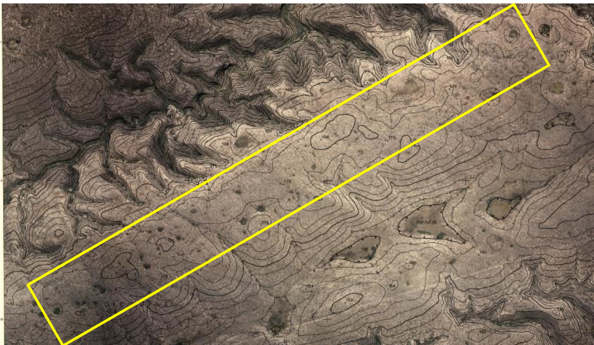
Figure 5. Topographic map of the Southern Plateau showing type A1 doline population – low density, isolated dolines on a sub-horizontal surface (within the yellow box, which is the yellow box in Figure 4). No doline can be seen on the slopes.
