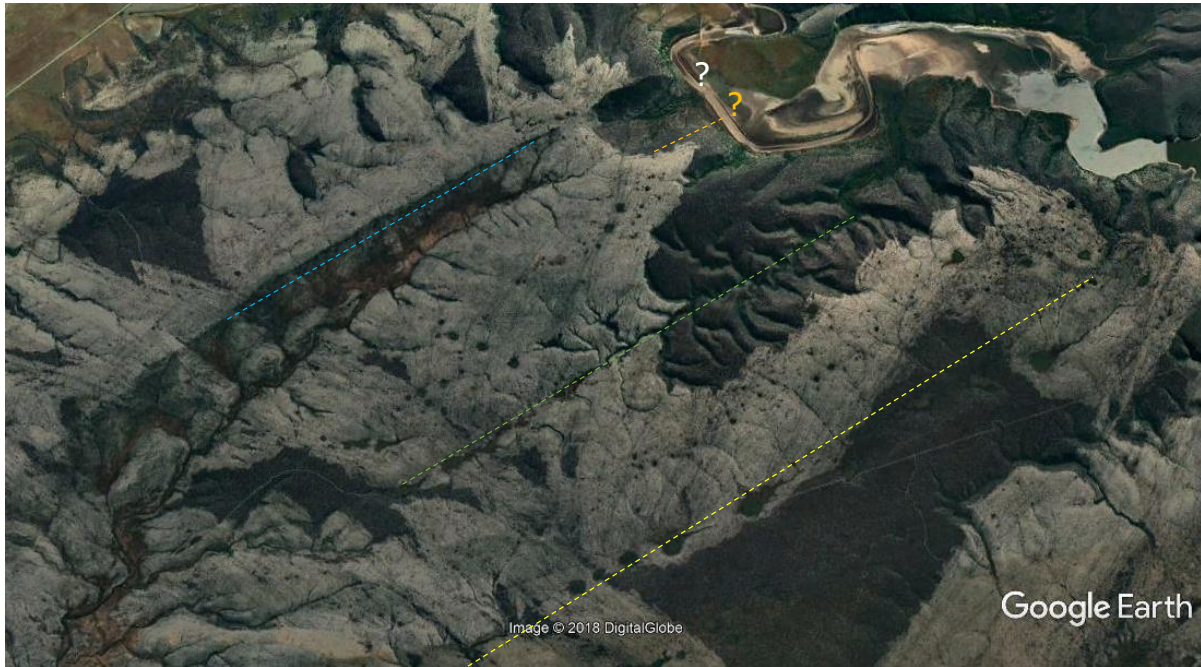
Figure 4. Satellite image of the area west of the Salt River Gorge, showing approximate locations of possible sub-parallel fault or fracture zones: white – Koleskloof North Wall Fault; ochre - Koleskloof South Wall Fault; blue – Patryze Fault; green – Langkloof Fault; yellow – Dolines Fault.
