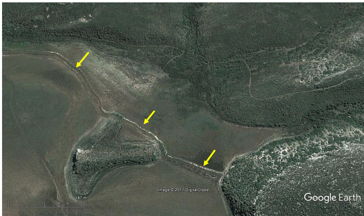
Figure 17. Satellite Image. When the water level in the marsh is low, the road is exposed on a low dyke above the marsh floor.
