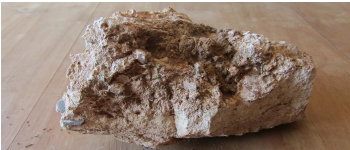
Figure 9. Calcrete on the Bokkeveld Bidouw formation shales: top - satellite image of an area north of the Soutpansvlakte Basin; the light patches (arrows) are calcrete; middle – a patch of disintegrated and broken (by farming machines) calcrete (note that the crop is shorter); bottom – a chunk of the calcrete (porous, compared with the compact calcrete on the Ceres Formation).
