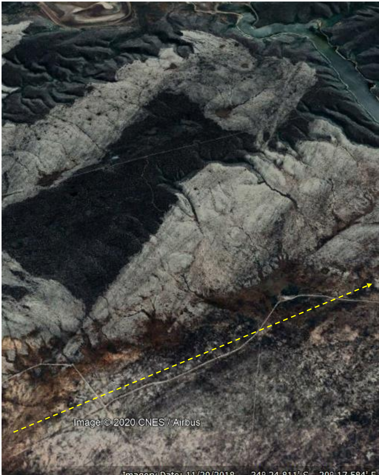
Figure 4. Satellite image of part of the Study Area, showing the Wankoe Formation (NW from the dashed line) and the Waenhuiskrans Formation (SE of the dashed line). The dark areas are calcrete surfaces covered with thick vegetation. The grey areas are calcrete surfaces, exposed after a bushfire. [The pink areas NW of the dashed line are the nonconsolidated sands of the Wankoe formation].
