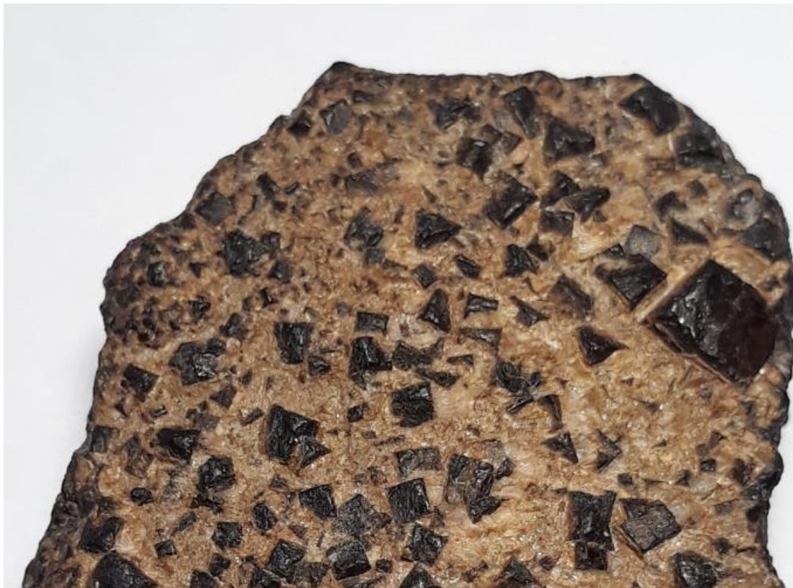
Figure 7. Top and bottom – cubic crystallisation of iron oxides (on Vinkelkop). Box in top photo enlarged in bottom photo.
