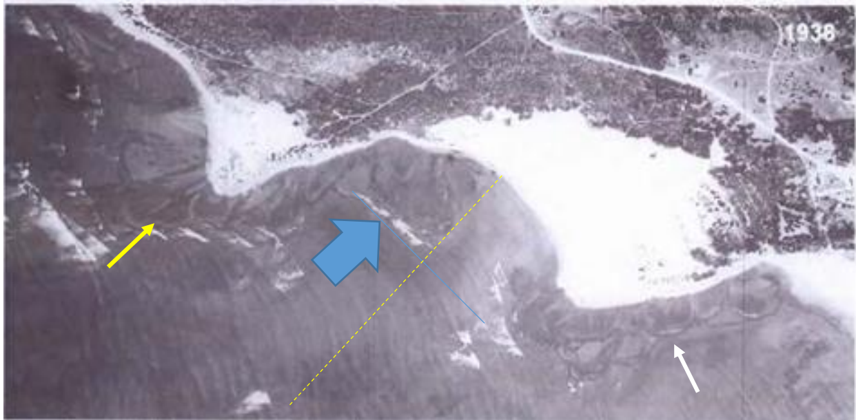
Figure 4. Oblique aerial view of Struis Bay in 1938. Trap clusters (white – western; yellow – eastern) can be seen through the water. The dashed line is the line along which the harbour wall was constructed. Blue arrow points to the area where sand was accumulated after the building of the harbour wall.
