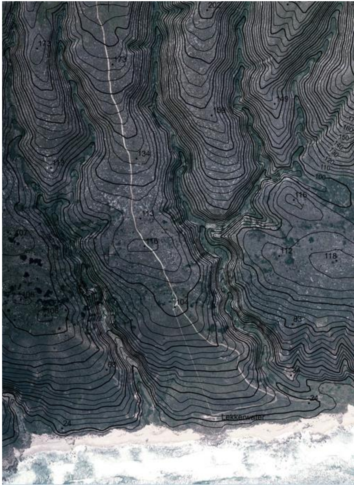
Figure 2. Topography map (1:10,000, contour interval 5 m) of Lekkerwater, showing the high relief of the area.
