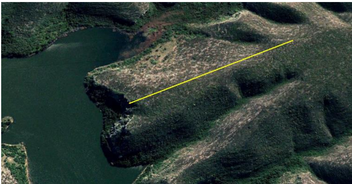
Figure 11. The assumed, general direction of the Guano Cave (length of the yellow line is the reported length of the cave – 656 m), wholly within the Wankoe Formation. The thickness of this formation over the entrance is ~30 m and 70 - 80 m over the far end of the cave.
