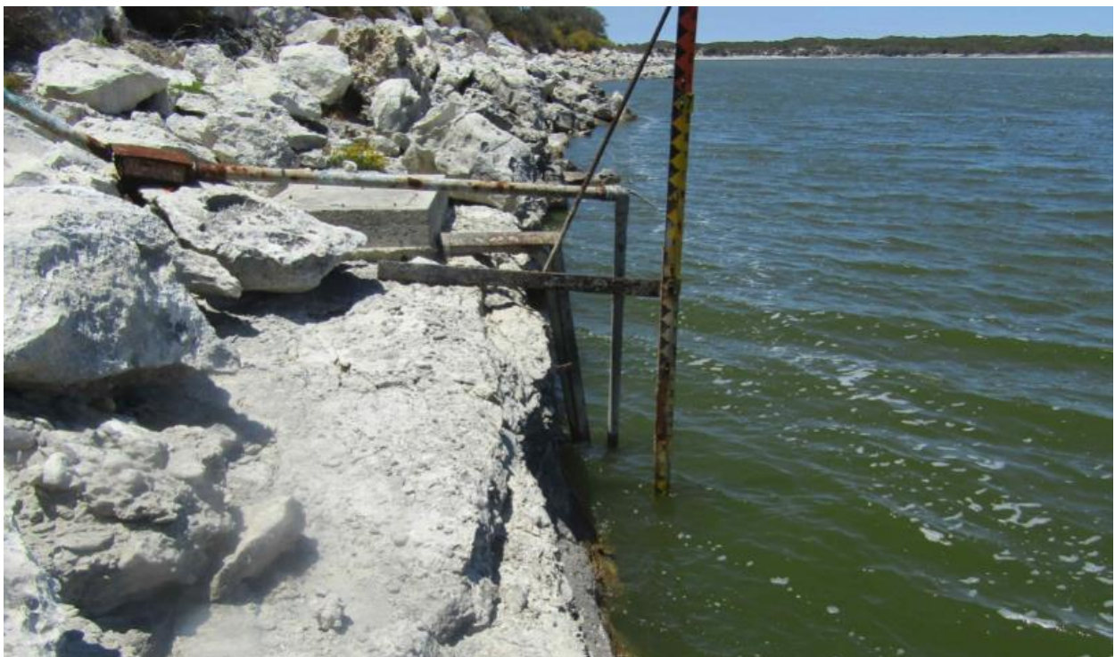
Figure 3. The hydrometer on the southeast shore of the De Hoop Vlei. The south shore of Die Mond can be seen at a distance.
