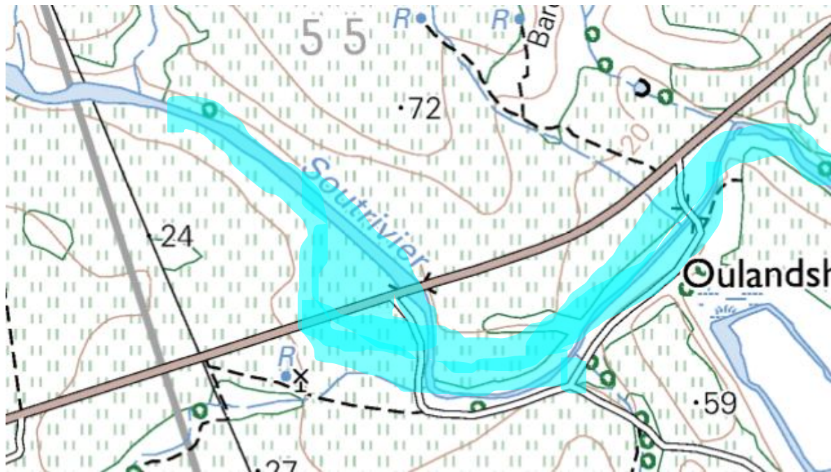
Figure 2. Blue paint indicates the approximate extent of the flooded road to Ouplaas. The water rose to ~17 m above sealevel, or ~2 m above the bridges in this map.
