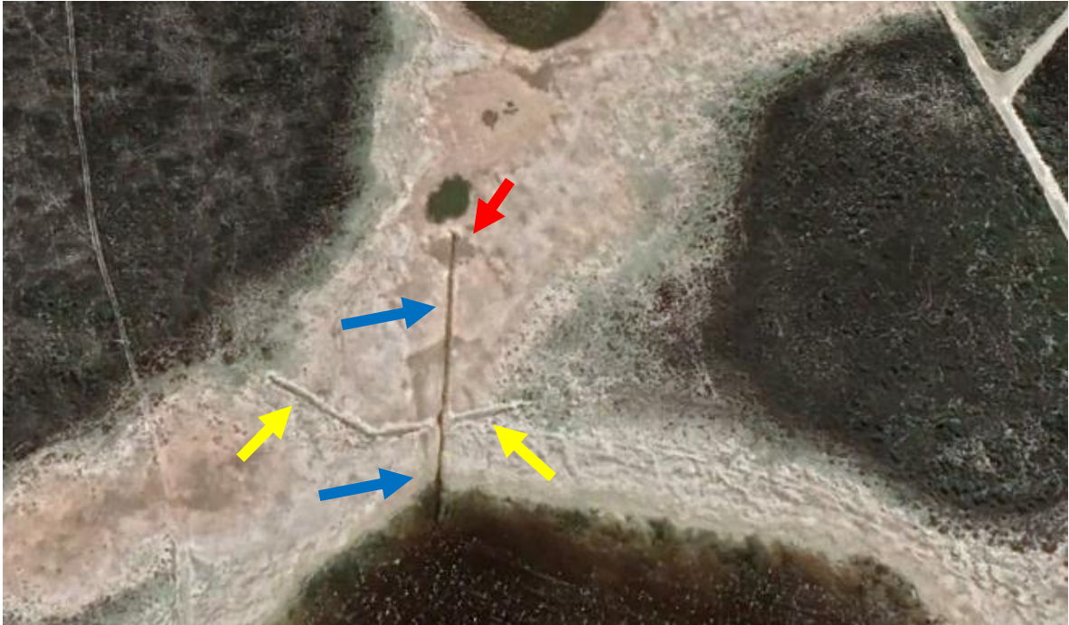
Figure 20b. Enlargement of the boxed area in Figure 20a. The low dyke (yellow arrows) and the canal (blue arrows) can be easily recognised. Red arrow points to a sinkhole (Figure 21).
