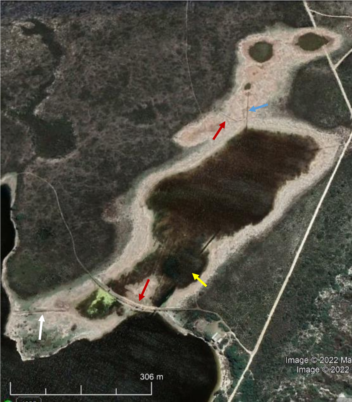
Figure 6. Satellite image of the features of the dam system in the Die Mond Depression. Arrows point to: white – front canal; yellow – middle canal; blue – back canal; red - dyke.
