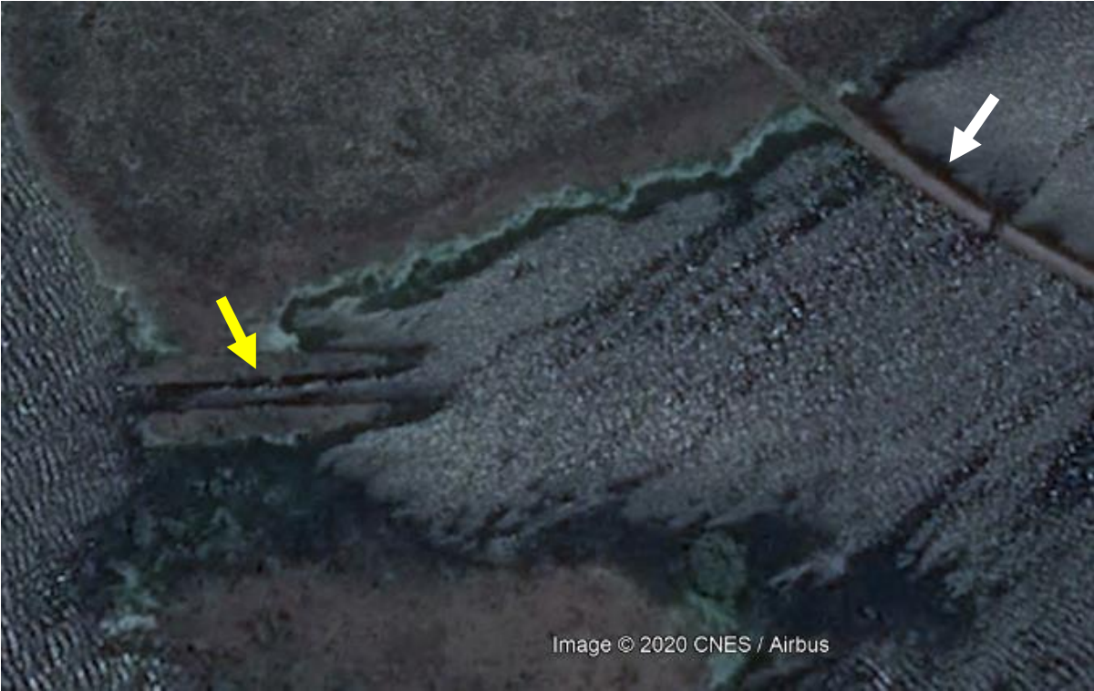
Figure 8. The canal (arrow) to the front doline is easily discerned when the depression is nearly totally flooded. White arrow points to the dyke.
