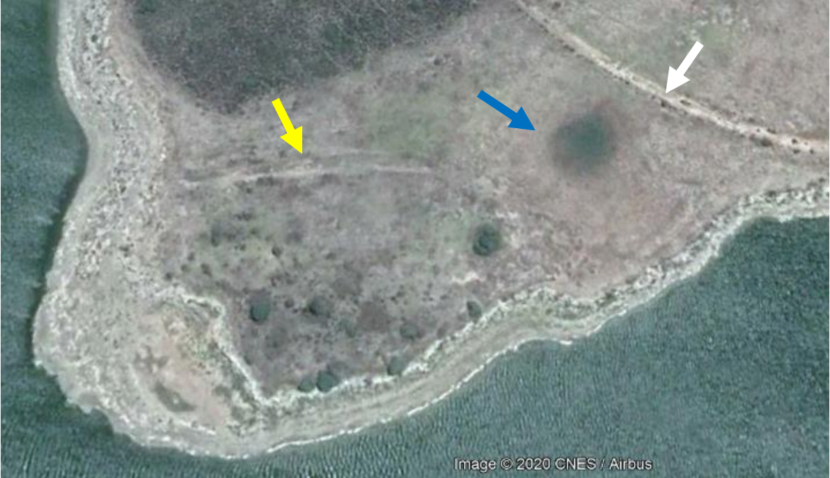
Figure 7. Enlargement of the red box in Figure 6. Yellow arrow points to the front canal, which delivered water to the front doline (blue arrow). White arrow points to the dyke.
