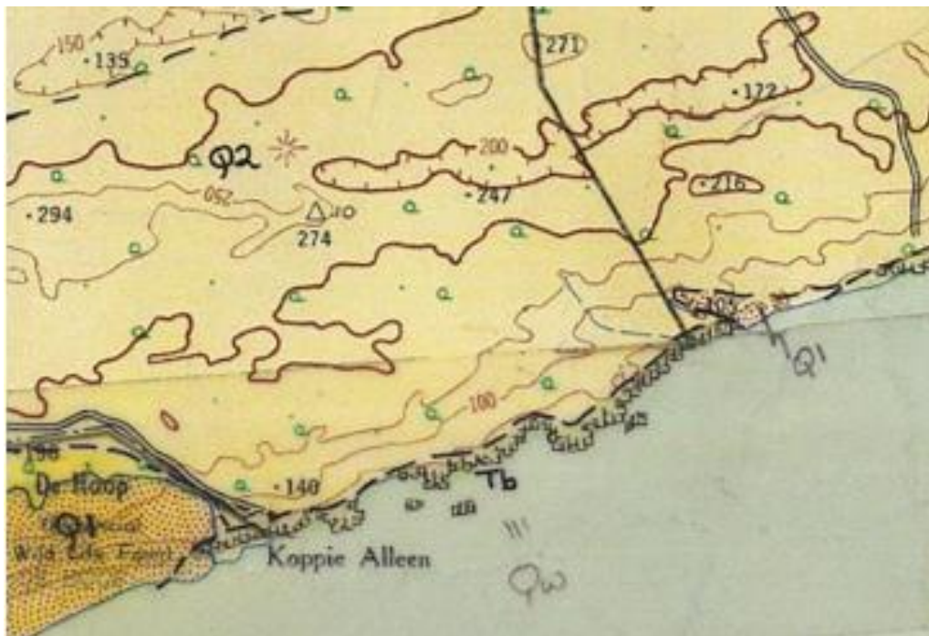
Figure 1. Koppie Alleen area. Top - Topography map (1:50,000). Bottom - geology field sheet (1:50,000, Malan 1984). Three formations of the Bredasdorp Group are present: dark green indicates the aeolianites of the Waenhuiskrans Formation; light green indicates Bredasdorp Group (undivided); Q1 and dotted areas indicates sands of the Strandveld Formation. Light yellow, and the Q2/Tb symbol indicate sediments of Quaternary over Bredasdorp Formation.
